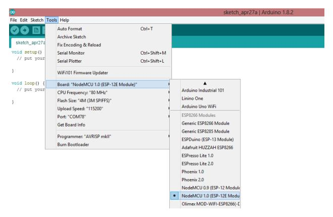
Launch ESP8266 Arduino IDE, Select Tools -> Board -> NodeMCU v1.0; and ensure parameters are correct. Refer to screenshot.
